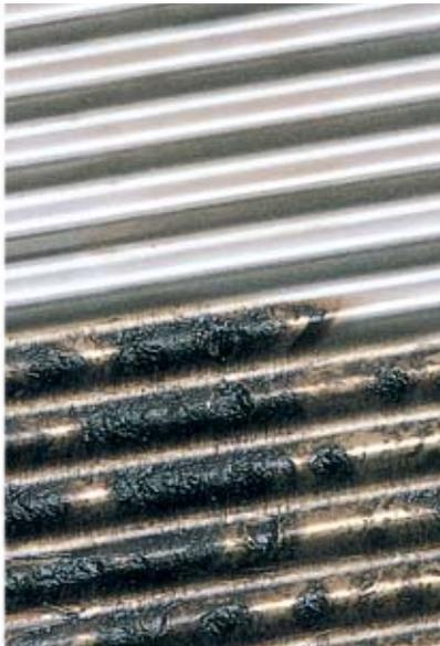
*Dirty plates affect heat transfer and reduce performance. Uncontrolled temperatures can affect the process, working environment and the product's quality. The upper part shows the result after cleaning.*
